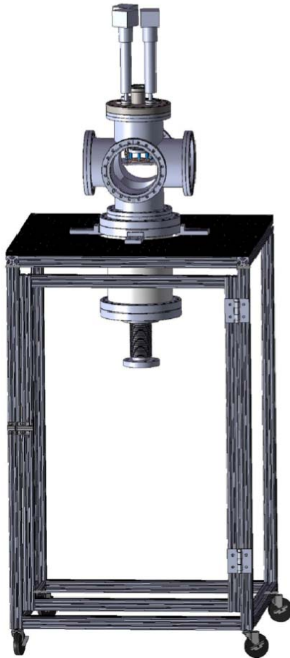
Figure 18. Complete cathode test cell assembly rest on the movable test stand. This will be the configuration used for experimentation. Note that the door will be interlocked and there are mesh screens in the test stand side panels.
